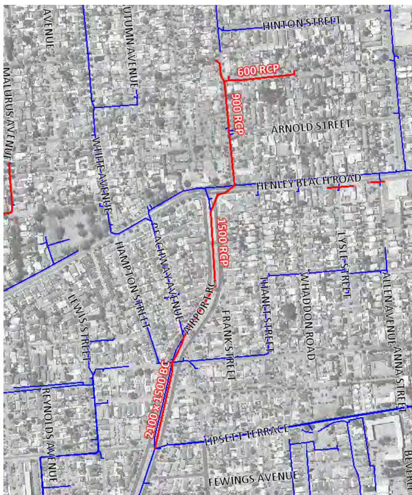
Figure 4.48 – Airport Road, Mellor Avenue Drainage Layout
