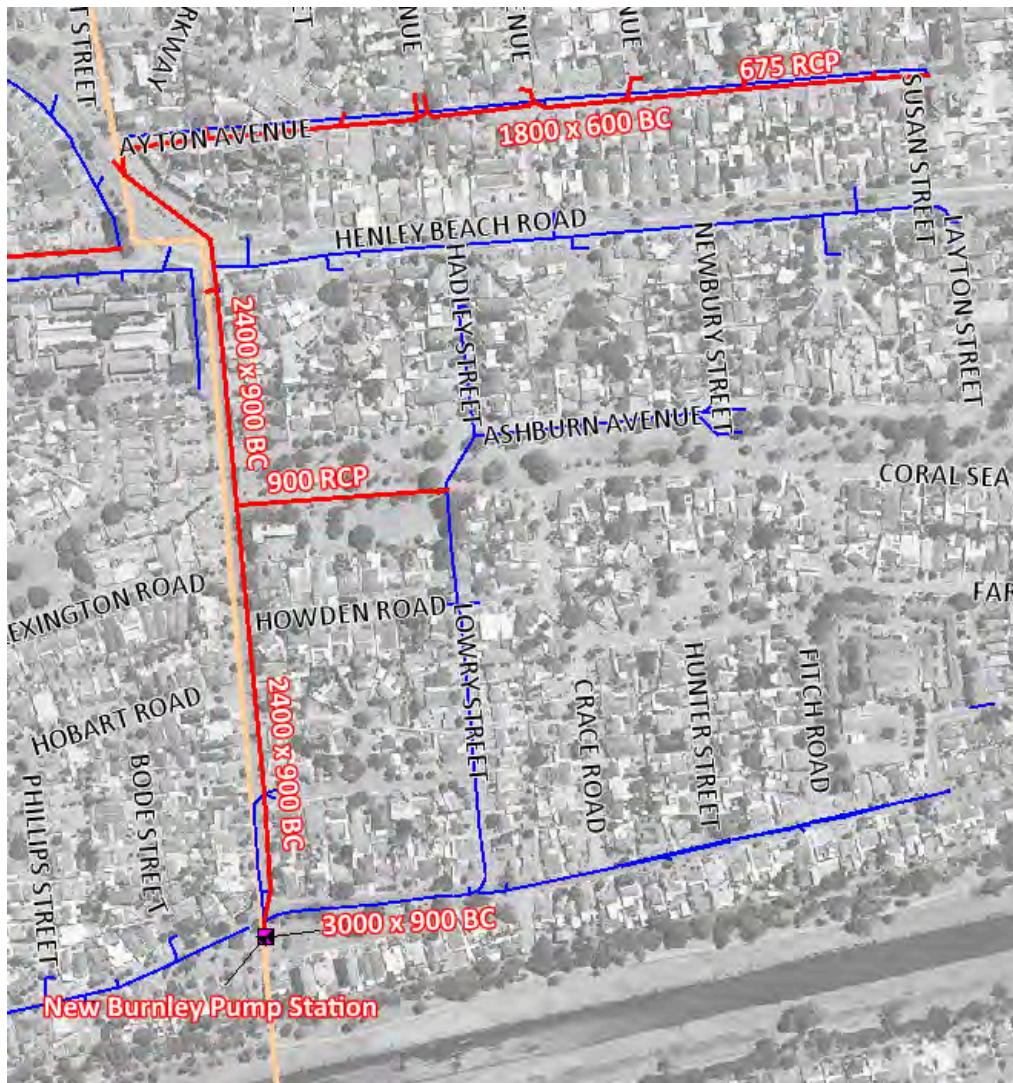
Figure 4.27 – Burnley Street Pump Station and Drainage Layout
