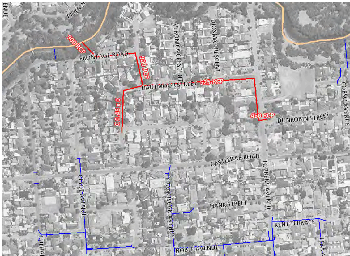
Figure 4.29 – Frontage Road Drainage Layout
