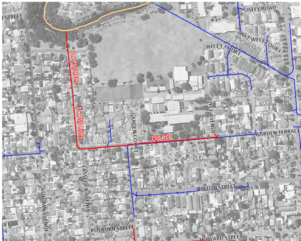
Figure 4.37 – Lasscock Avenue Drainage Layout
