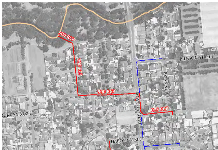
Figure 4.31 – Matt Street Drainage Layout
