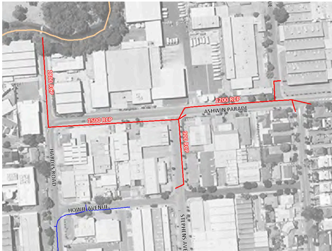
Figure 4.40 – Ashwin Parade Drainage Layout
