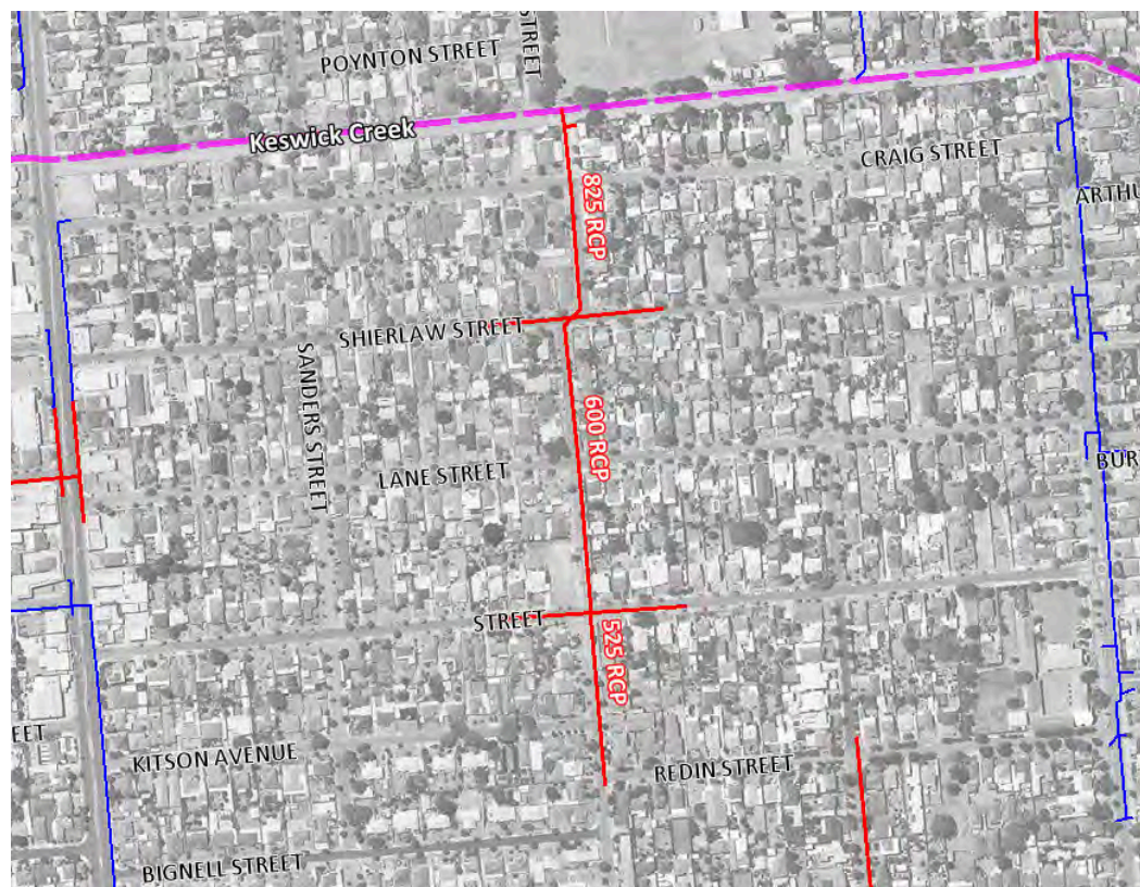
Figure 4.58 – Chambers Avenue Drainage Layout
