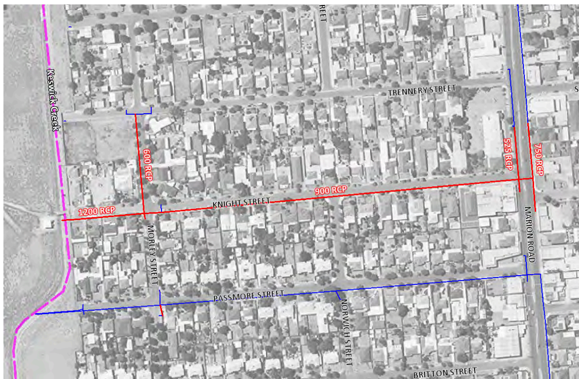
Figure 4.59 – Knight Street Drainage Layout
