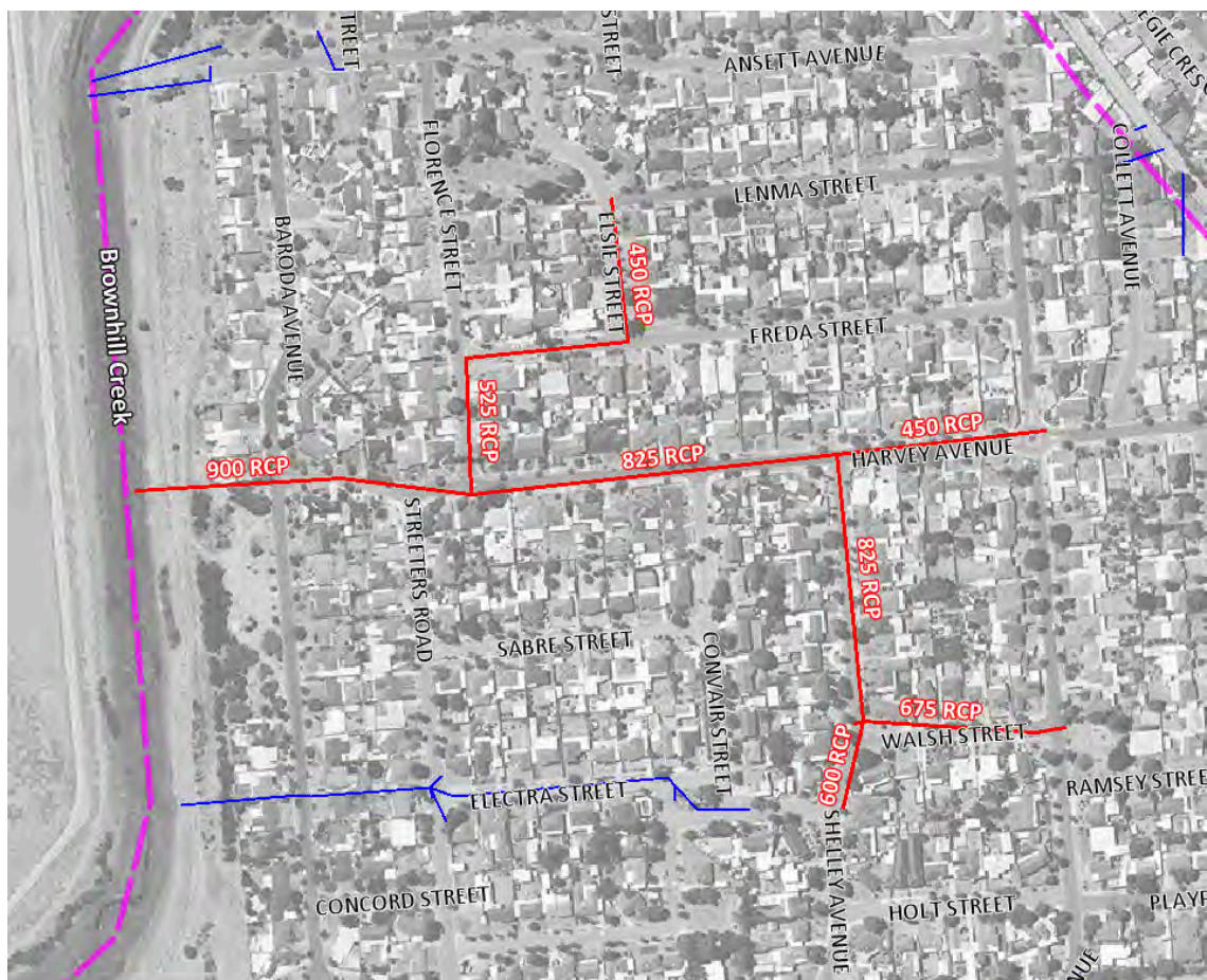
Figure 4.66 – Harvey Avenue Drainage Layout
