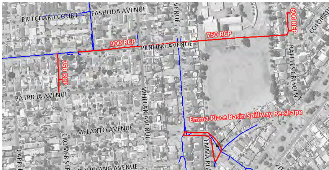
Figure 4.74 – Penong Avenue Drainage Layout
