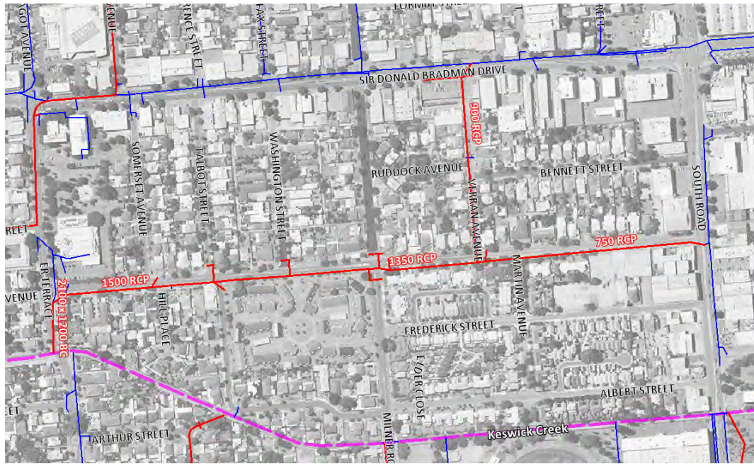
Figure 4.51 – Davenport Terrace Drainage Layout
