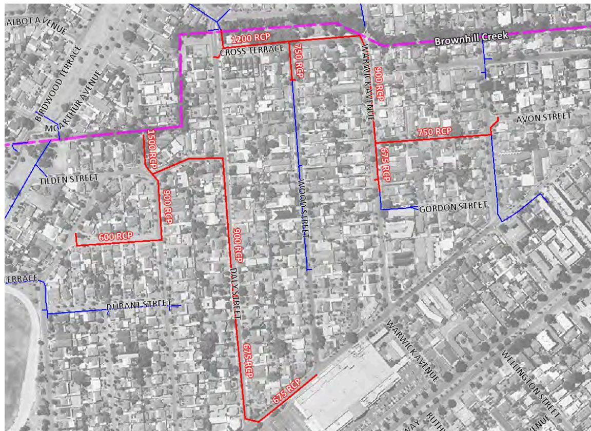
Figure 4.64 – Warwick Avenue and Gray Street Drainage Layouts
