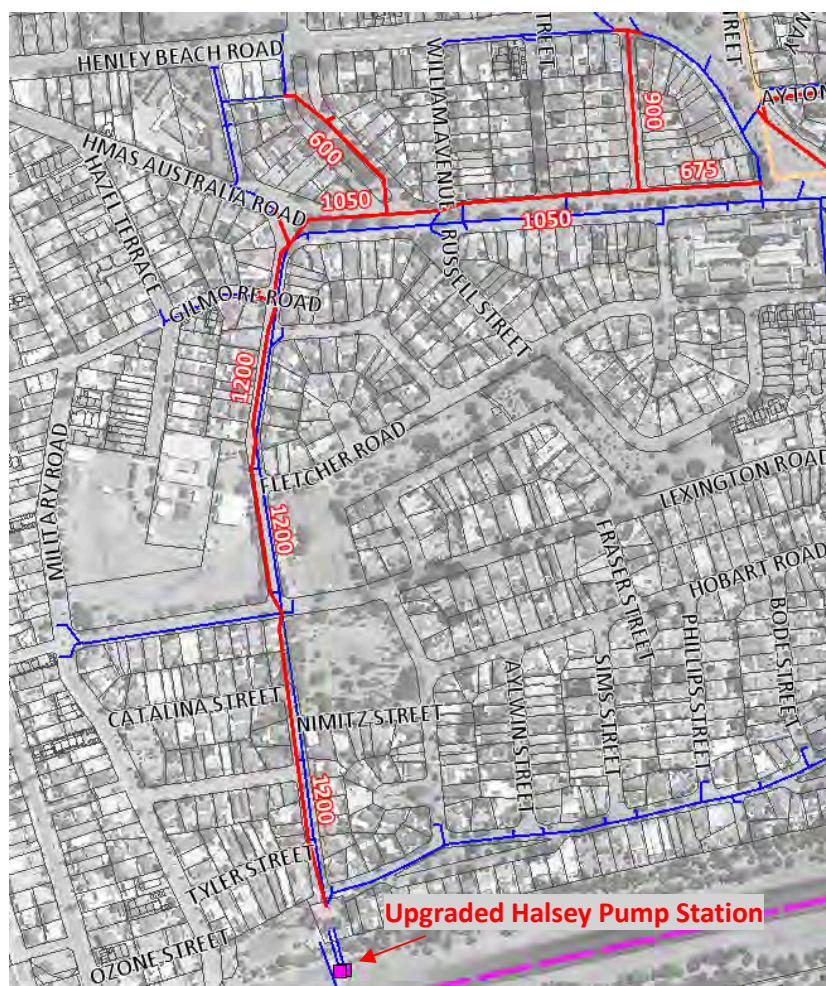
Figure 4.26 – Halsey Pump Station and Drainage Layout
